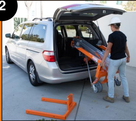
2 Fold and pin legs so they will clear opening.
