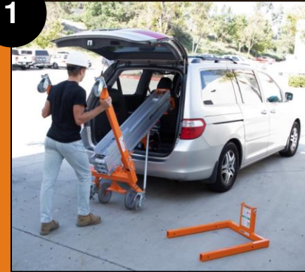
1 Remove forks and lean machine back into van under lift gate.
